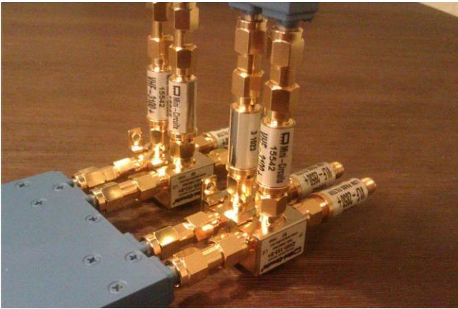
Figure 2 - 4 channel RF-mixer with 1:4 port divider, HP and LP filters
