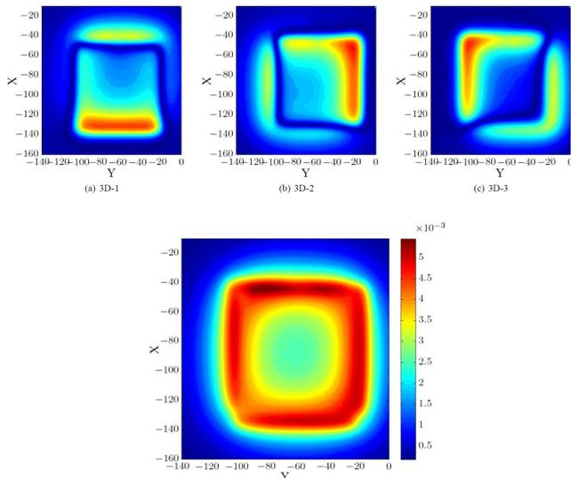
Figure 6 - H-field results obtained at 5 MHz, a/b/c/ are the individual readings from the orthogonal H-field rod antenna, the lower figure yields the composed result.
