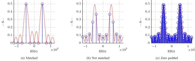
Figure 5 - Influence of FFT mapping on spectral plot
