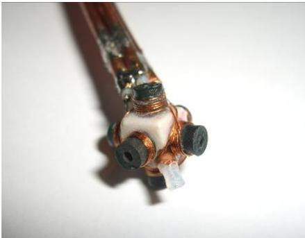
Figure 3 - Photo of the orthogonal 3 axis H-field probe
